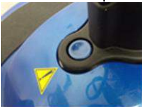
Tiller Lock in un-locked position:
